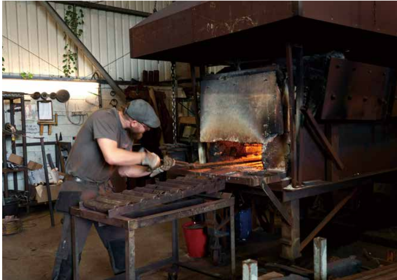
Above: Forging wrought iron at Topp & Co., in the suburbs of York in northern England.
