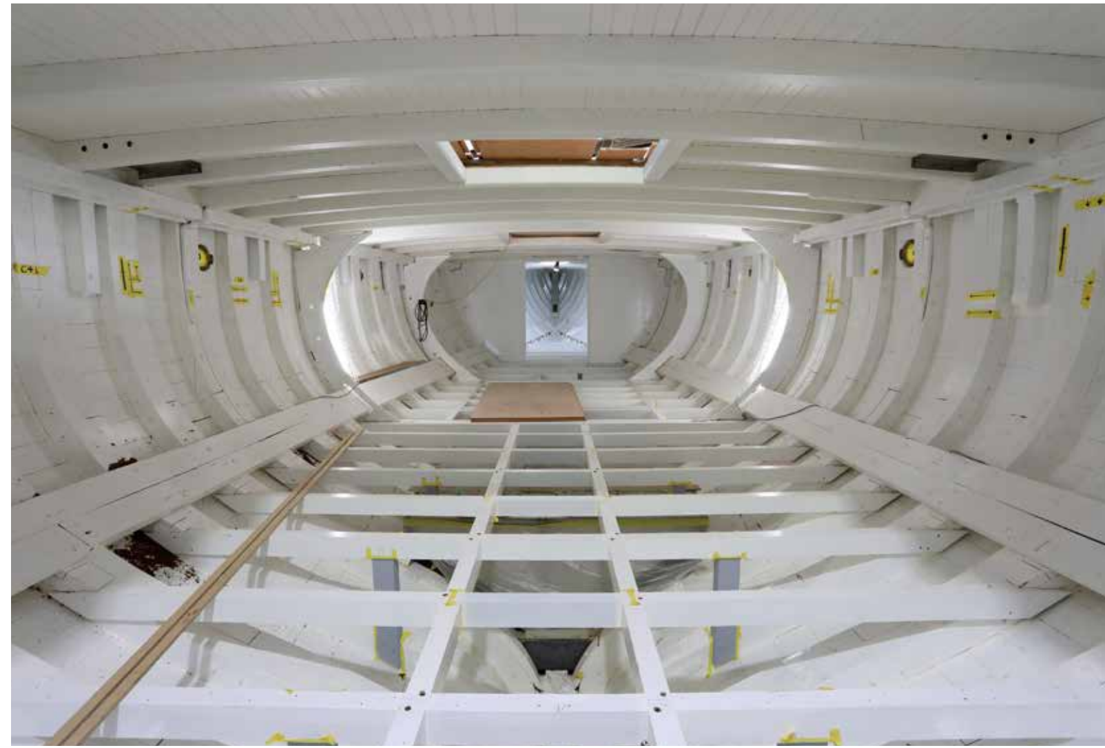
Above: August, 2019. The interior of the hull construction from stern to bow. A water tank is set into the hull, on top of which are the beams that will support the wooden plank flooring. Below: Riviera Group Chairman Noboru Watanabe, surrounded by the Cynara restoration team. Leading the team are Paul Harvey (far right) and Ben Hobbs (to the right of Watanabe). On the far left is project manager and restoration expert Feargus Bryan.
