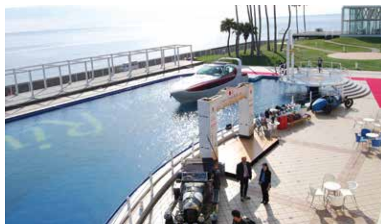
Right, YANMAR X-39 Tonnage: 7,200kg Overall length: 11.8m Width: 3.0m Engine: YANMAR Horsepower: 370hp x 2
